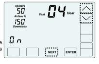
Maximum Allowable Downstairs Airflow in Heating
