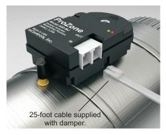
The damper has an RJ11 connector to connect the damper to the panel using the 25-foot cable provided with the damper. A second RJ11 connector is used to daisy chain two or more dampers in the same zone.
