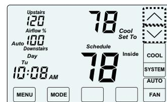
Touch the UP/DOWN keys to adjust the setpoint temperature.
