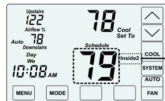
To display the upstairs temperature, touch the INSIDE temperature as indicated. The thermostat will now display the upstairs temperature, indicated by INSIDE2.
