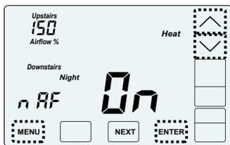
Touch the **MENU** key to display NIGHTTIME, UPSTAIRS AIRFLOW IN HEATING indicated by nAF Heat.
